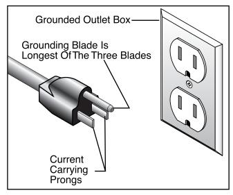
**Figure 1.** NEMA 5-15 plug and grounded outlet.
